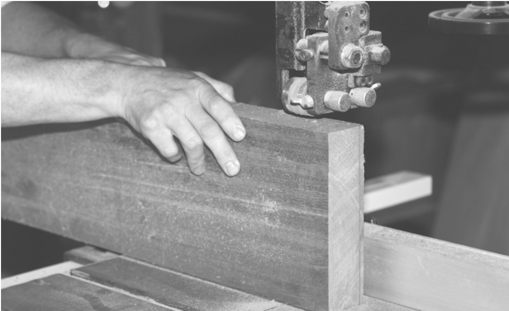
(Photo 1-2) Resawing thick stock to make back plates. Each will be sawn to make ample thickness for joining the back halves and sanding out all of the saw marks. Saw the back plates and tops to a minimum thickness of \frac{1}{4} inch to allow joining and final sanding.
