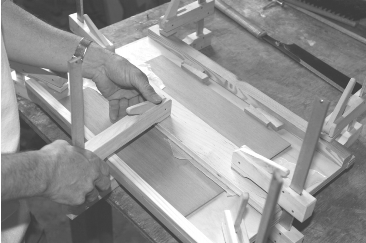
(Photo 2-3) Plate Gluing Jig. Notice the small wooden wedges at the back and the caul across the center seam. The two extra clamps in the front corners are just used to keep the bottom board level.
